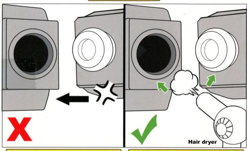
Do not assemble the parts directly without soften.
